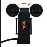
Wait for the end of the charging process. The unit is fully charged when the red LED goes out, see "1.11 Meaning of the LED lights" of this manual.
